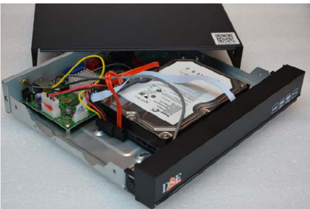
Secure the hard disk with the 4 screws provided that screw tight from underneath the VCR
