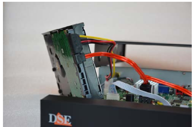
Connect the hard drive with the two power and data cables you find inside
